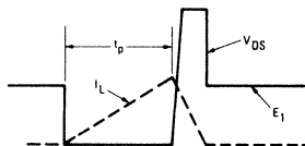
Fig. 16 -- Clamped Inductive Waveforms
